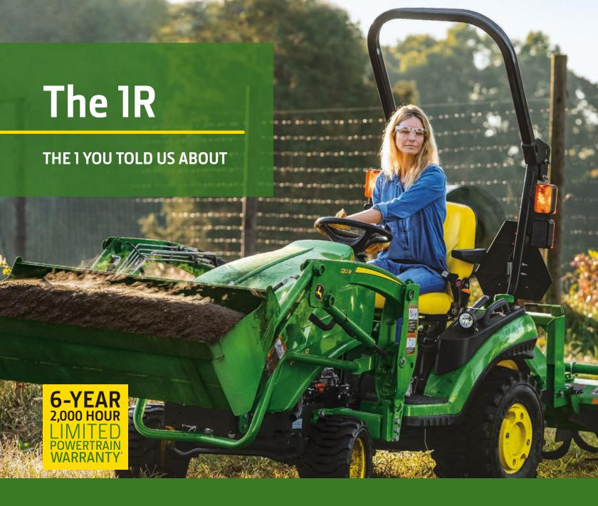
We asked sub-compact utility tractor owners during development, "what would the best small tractor look like to you?" The answer? This 1, the 1025R. The 1025R has a 23.9 HP² (17.8 kW), three-cylinder diesel engine that delivers responsive, efficient horsepower in just about any application. Everything from clearing a sidewalk or a driveway of snow to mowing an acre of lawn to digging out a water feature or drainage ditch.
