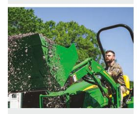
THE 120E LOADER is our most affordable loader option and is non-self-leveling (NSL). The lift capacity is 519 lb. (236 kg) measured at 500 mm ahead of pivot<sup>3</sup> with a max lift height of 71.2 in (1809 mm).
